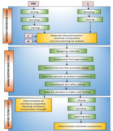
Fig. 2. Flow diagram of the experimental program stages
