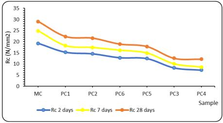
Fig. 6. Average compressive strengths at 2, 7, 28 days
