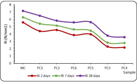
Fig. 5. Average bending strengths at 2, 7, 28 days
