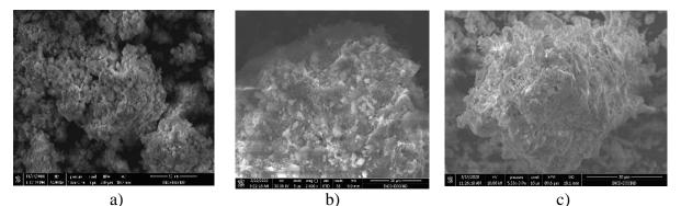
Fig. 3. The SEM images for the three component materials of the mortars, a) red mud NR, b) mine tailings S, c) cement C
